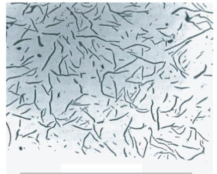
The micrograph shown in the second image above illustrates the flake composition of grey iron. The first image shows the micrographic of the nodular graphite in ductile iron.
